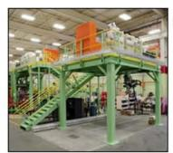
Utilize Mezzanines ... to increase square footage without bricks and mortar. In buildings with sufficient ceiling height, mezzanines elevated above the floor make use of unused overhead space to provide 2<sup>nd</sup> and 3<sup>rd</sup> level storage of shelving, case flow or pallets. Total pick faces can be doubled or even tripled with effective use of storage mezzanines.
