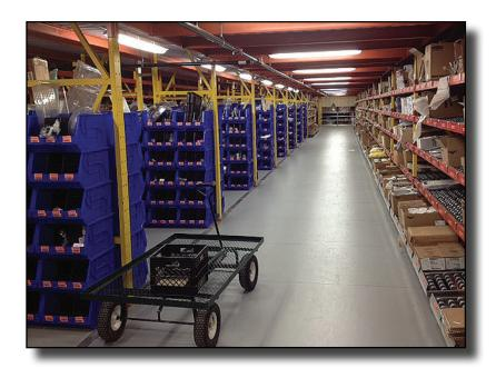
New pick module helped Martin Bros. achieve far greater item density in a small facility footprint; 40 slots per 5-high, 8-wide carton flow bay and up to 196 slots within the tote section, resulting in a dramatic increase in pick rates.
